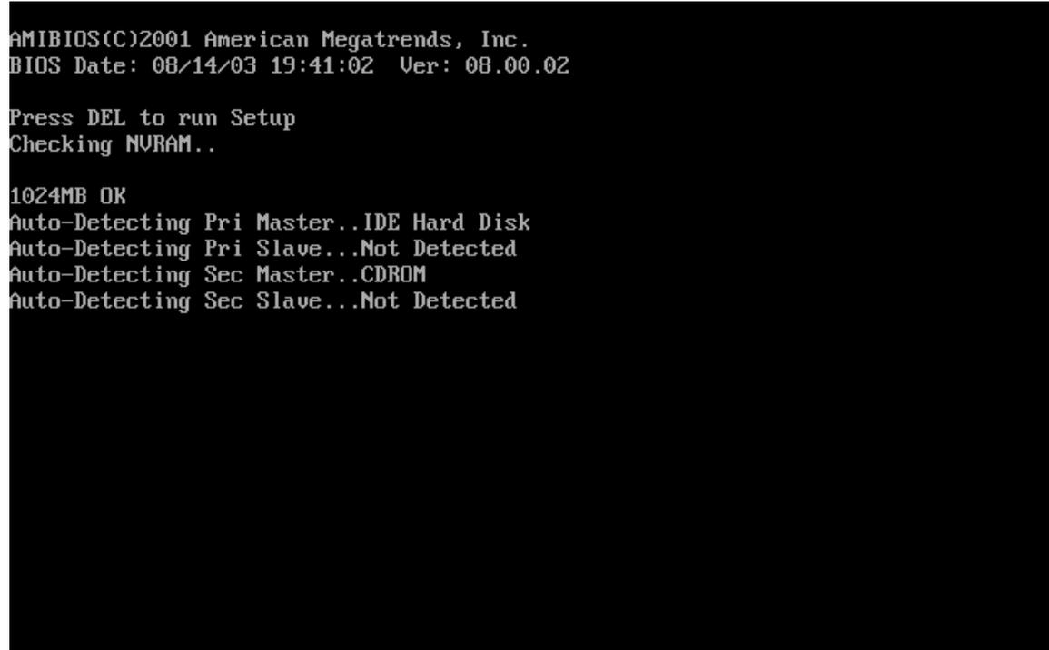
A screenshot of a computer's BIOS POST screen. The text is white on a black background. It shows the BIOS version and date, a prompt to press DEL for setup, and the results of a memory and hardware check.
