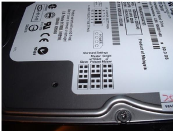
Move the Master/Slave jumper on the installed hard disk drive to the Master position if it is in any other position.
